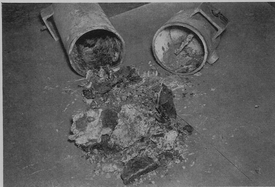
Figure 2. Sprayer tank failure due to corrosion
